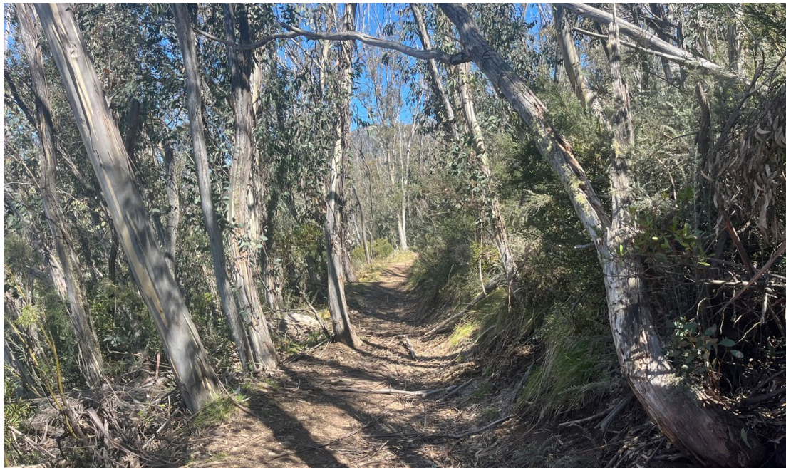
Figure 12: Example of Sidewinder trail within the native vegetation. The fallen leaf litter/debris protects the trail tread during winter. Evident erosion is better managed through natural features vs treeless disturbed ski slopes. Photo taken 10 October 2023.
